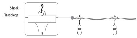
**3** Attach each plastic loop to the guide wire.
