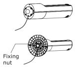
Place the assembled base to the bottom of the fan body by aligning the matching holes, and fix them together. Then fit the base with screws.
