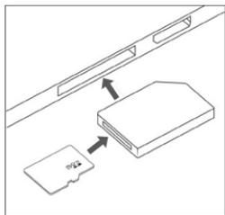
To playback a video using an SD card adapter, remove the memory card and insert it into an SD card adapter. Place the adapter in the computer.
