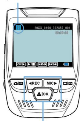
During playback use the OK (pause), MIC (fast forward) and REC (rewind) buttons to control the video playback.
