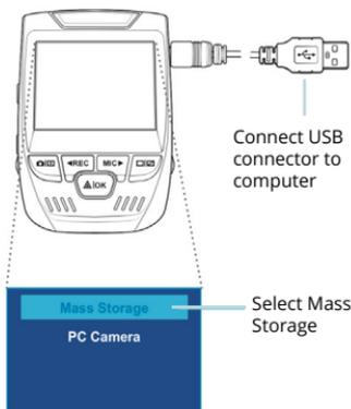
After the device powers up, press the OK Button to select Mass Storage. On the computer, navigate to device drive. The videos are stored at: \CARDV\ MOVIE.
