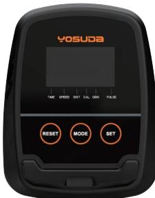
**RESET:** Press to reset time, distance, and calories. Short time press will turn the value of the current MODE to 0. Extended-press will turn all values to 0 except ODO MODE. If you need to reset ODO, please take off the battery and install it again.
