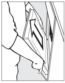
■ Hold the door on either side and pull it upwards off the hinge retainers.
