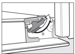
Release the locking clamps by turning them as far as they will go. You could damage the oven if you remove the door incorrectly.
