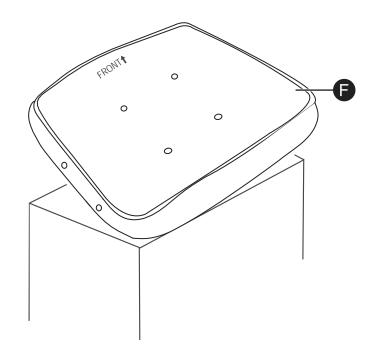
5 Align the riser mechanism (E) on the bottom of the seat (F) and attach it to the seat with four  $5/16" \times 3/4"$ screws (K). Tighten the screws with the Allen wrench (J).
