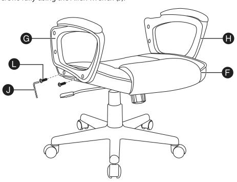
**8** Attach the arms to the seat back (I) with four  $1/4" \times 1"$  screws (L) and tighten the screws fully using the Allen wrench (J).
