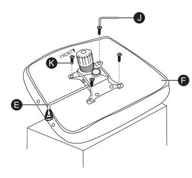
6 Lift the seat bottom (F) and turn it right side up, then align the hole in the riser mechanism (E) with the center support post (C) and press the seat down until it clicks into place.
