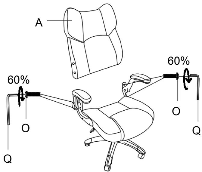
Tighten the screws to 60% first, and then tighten the screws to 100% after all screws are fixed.
