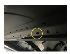
Pass the new windshield washer hose through the visor ROPs and connect to the black side of the check valve.
