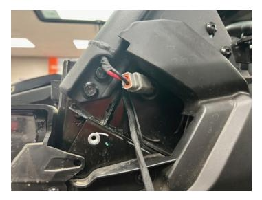
Pass wiring up over steering column toward center of vehicle. Keep wiring away from moving objects in the steering wheel / pedal area.
