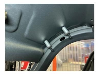
Reinstall the (3) T40 Torx bolts and 15mm nuts previously removed from between the roof and ROPs support.
