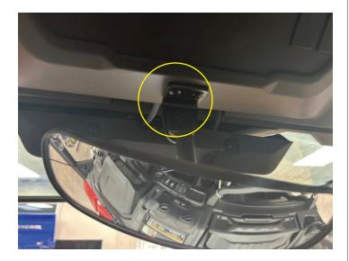
• Remove (6) T27 Torx screws from OEM visor (if equipped).
