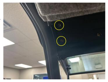
On center OEM bracket - carefully remove and disconnect wiring and windshield washer hose.
