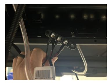
Attach the Buss Bar to the top of the ROPs visor as shown with a M6 x 14mm bolt and M6 Nylock Nut.
