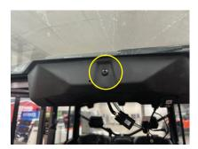
Remove the windshield washer hose clamp with a pliers. (You will re-use the clamp and check valve in later step.)
