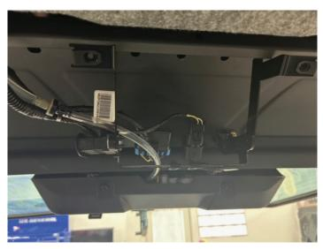
Remove (4) T30 Torx bolts and 10mm nuts from center bracket.
