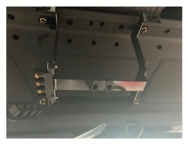
Remove windshield washer motor cover with (3) T30 Torx screws. (Allow cover to hang or unplug wiring and remove.)
