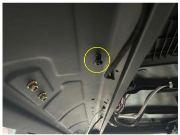
Install the visor using M6 washers and M6 Nylock nuts.
