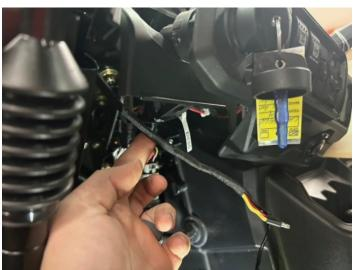
Connect Acc T-Harness into the 2 pin connectors below the buss bar. Then connect the bullet connector from the T-Harness to the A-Pillar harness.
