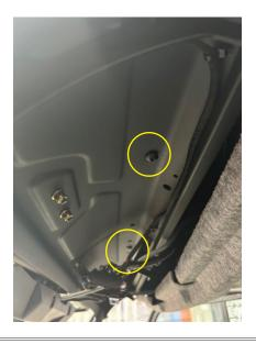
Remove OEM driver side visor bracket using a T30 Torx and a 10mm wrench or socket.
