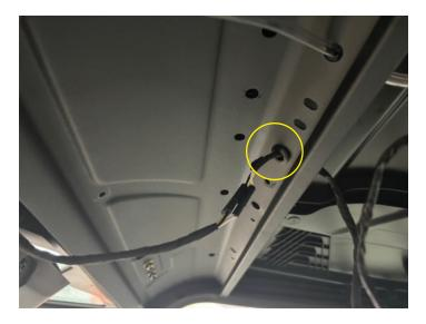
• Connect the three pin Weather Pack connectors together.
