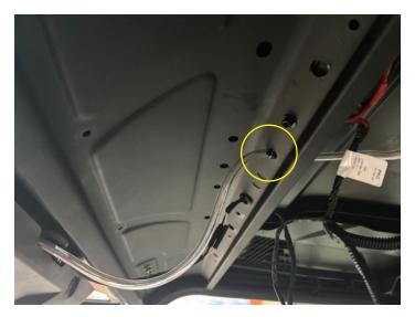
Pass windshield washer power extension harness through ROPs and connect bullet connectors.
