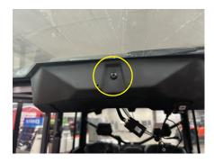
• Defender Limited ONLY: Relocate power harness through ROPs hole as pictured.
