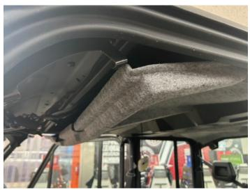
Remove (3) T40 Torx bolts using a 15mm wrench on the topside between the bracket and roof to hold the nut. (Two bolts circled, the passenger side is the same as driver.)
