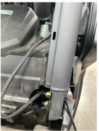
• Carefully tuck the wiring harness behind the foam strip at the front of the dash.
