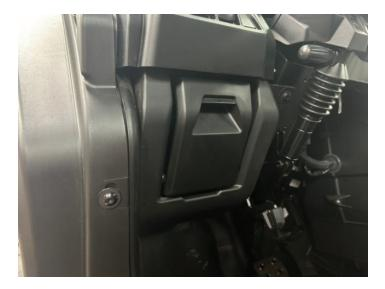
• Remove center switch panel by pulling out from the top edge.
