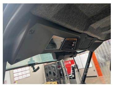
Remove a T20 Torx screw on driver side headliner (if equipped).
