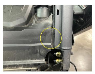
Pass A-Pillar harness wire through grommet to the inside dash area. Reach your hand up through driver side pocket area to help.
