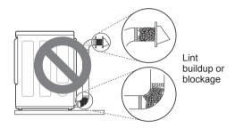
Make sure the ductwork is not crushed or restricted.
