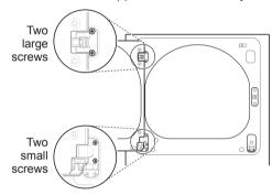
While supporting the door, install the two small hinge screws removed in step 2. Test the swing of the door to make sure the hinges and latch are properly aligned and that the door opens, closes and latches properly in both directions.
