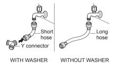
Connect all water supply hoses tightly by hand and then tighten another 2/3 turn with pliers.
