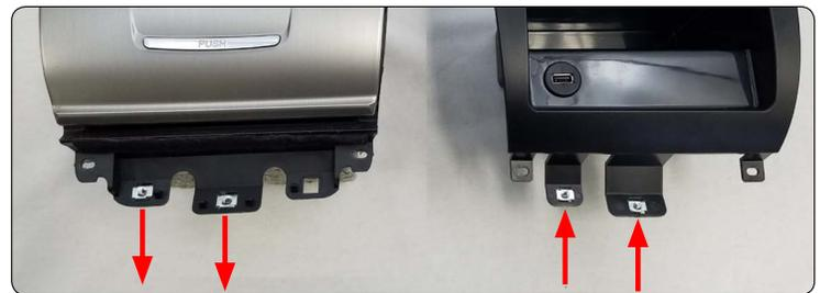
3. Install the pocket into the dash by sliding it back until the clips lock into the openings in the dash. Secure it using the two phillips head screws removed in step 1.7.
