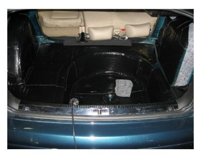
We recommend 100% coverage is recommended for optimum acoustic performance of the trunk area. The space from the rear well to the driver/passenger is a determining factor. The shorter the distance the greater sound transmission and annoyance factor from road, tire and aftermarket exhaust noise.
