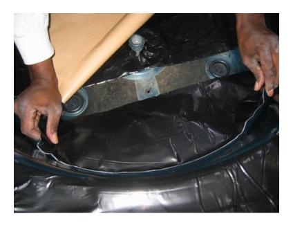
Repeat the above step until you have covered the floor and rear wall of the trunk. A good tip is to save any small cut outs or pieces of the HushMat Ultra for patching smaller areas of the trunk. For example if you cut around the top radius of the wheel well save the cut piece and place it on the floor pan in the wheel well as this will be the same radius.
