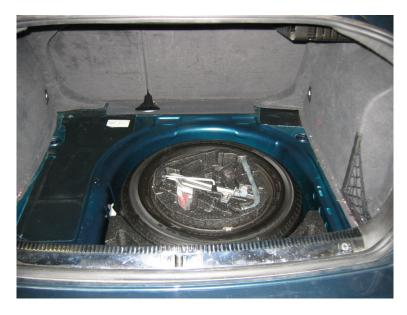
Remove all plastic and fabric trunk trim and spare tire (on many vehicles you may be required to remove the rear seats in order to effectively reach these areas). Vacuum loose dirt, sand or dust from the sheet metal surfaces.
