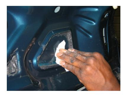
Wipe up any excess material within 15 minutes with a water soaked rage. Flush out the nozzle with water for re-use. If the tube is not empty allow the tube to self seal and it can be used again. Allow 3 hours for the Ultra H-2-O to cure and you can sand and paint the lid if necessary.
