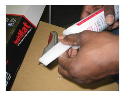
Cut the end of the Ultra H-2-O tube nozzle and screw on the EZ squeeze HushMat applicator nozzle. Place the tube into a standard  $1/10^{th}$  gallon caulk gun squeeze our any air in the nozzle.
