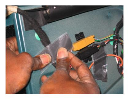
Place the cut strips over the wire and press the tape onto the vehicle surface. HushMat Quiet Tape adheres to sheet metal, plastic and fiberglass surfaces. Quiet Tape is a butyl rubber formula that maintains adhesion from -30 to 300 F.
