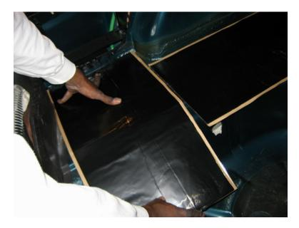
Prior to removing the brown release paper, place the sheet of HushMat Ultra damping material across a straight edge of the trunk beginning against the quarter panel wheel well of the vehicle to determine adequate fit or "nesting". Cut the sheet to fit the space, if necessary with scissors or utility knife prior to peeling back the release paper.
