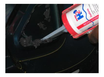
Apply a bead of Ultra H-2-O between the trunk lid frame and the outer skin – ensure that you have good contact on both surfaces with the H-2-O.
