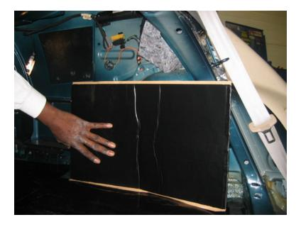
A major source of sound transmission in vehicles is through the rear wheel wells. The sheet metal continues to get thinner and thinner and sound transmits directly through into the vehicle interior. High performance vehicles, sub compacts, compacts and vehicles built low to the ground have extensive issues in this area. We recommend coverage of 100% of the interior side well Measure the sheet against the well while the brown release paper is still intact and cut if necessary.
