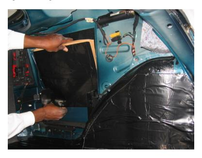
Treatment of the rear quarter panels is required due to the thin gauge sheet metal and the small amount of interface with the vehicle frame. These expansive panels are loosely supported and resonate. Cut the large sheet of HushMat Ultra in half and press it onto the inside of the outer quarter panel skin through the frame.
