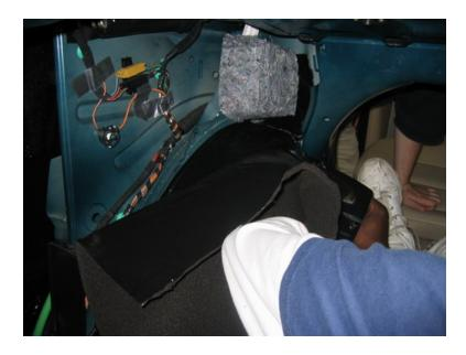
Lay the single sheet of HushMat Silencer Megabond over the wheel well with the white release paper intact. Measure and cut with scissors or utility knife. Peel back one straight edge of the white release paper and adhere the Silencer Megabond directly on top of the HushMat Ultra on the Wheel Well. Repeat this step for both wheel wells.
