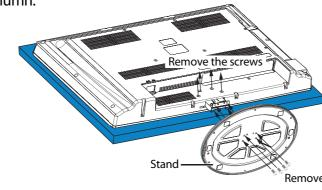
4 Attach the wall-mount bracket to your TV using the mounting holes on the back of your TV. See the instructions that came with the wall-mount bracket for information about how to correctly hang your TV.
