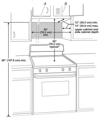
A. 2" x 4" (50.8 mm x 101.6 mm) wall stud B. Grounded 3 prong outlet
