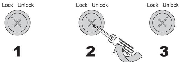
**Note:** The position of the lock button has molded in indicator dimple. When this is closest to the molded “Lock” the child resistant door is enabled. After it has been rotated it will be closest to “Unlock”, in this position the child resistant door is disabled.
