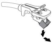
3 Insert the new stylus upwards into the slot under the head, then push upward until the tip locks into place.
