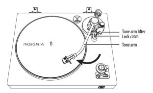
**5** Turn the counterweight so that the tone arm is horizontal. You can move the counterweight forward or backward on the tone arm.
