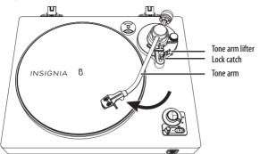
7 Push the tone arm lifter backward to lower the tone arm so that the stylus touches the record and starts to play.
