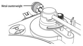
7 Hold the metal counterweight to keep it from moving, then carefully rotate the front black number ring so that 0 is in the 12 o'clock position.
