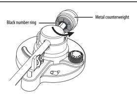
8 Hold both the metal counterweight and black number ring together. Rotate them counter-clockwise one full circle, then set the ring to 0.5 so that 0.5 on the dial is in the 12 o'clock position. This set the tone are to  $3.5 \pm .5$  grams of downward force (the recommended tracking weight) for this needle.
