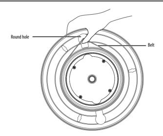
2 Still holding the belt, flip the platter over, then insert the platter onto the spindle in the center of your turntable.
