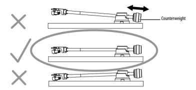
6 Hold the metal counterweight at the back of the tone arm.
