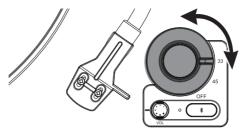
4 Remove the tone arm-rest lock catch to release the tone arm.
