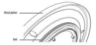
1 Make sure that the belt is not twisted, then use your thumb to stretch the belt until it reaches the round hole in the platter.
