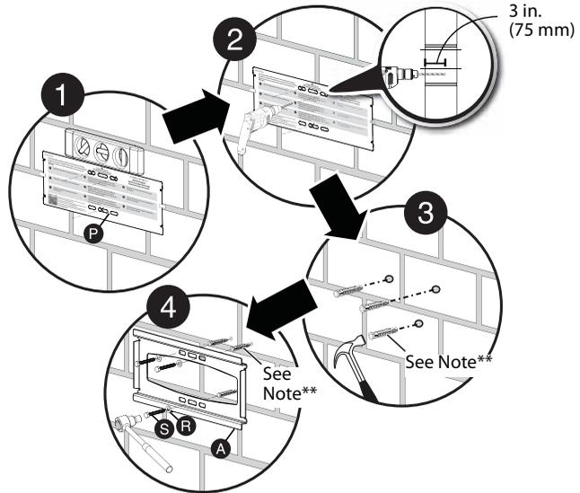
\*\* Note: Not included. Call Customer Service to have the Fischer UX 10 x 60 concrete anchor kit shipped directly to you.
