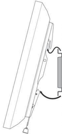
Pull bottom away from wall, then lift off the wall bracket.
