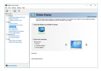
The display can be also rotated by selecting **Rotate Display** under the **Display** menu in the **NVIDIA Control Panel**.
