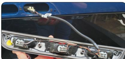
b. Place the third brake light onto the third brake light camera bracket and line up the screw holes.
