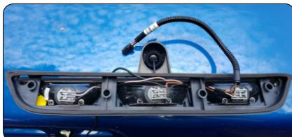
c. Reconnect the third brake light to the factory connector.
