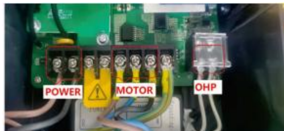
Single-phase Wiring (Actual Picture)
