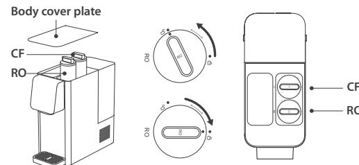
**Step 1:** Open the body cover plate as shown in the figure, and rotate the RO filter counterclockwise by 90 degrees to take it out.
