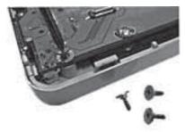
6 Insert the tab from the top of the enclosure into the slot and snap the lid into place. Then slide the switch to the locked position.
