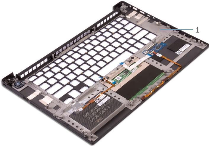
**Figure 37. Removing the palm-rest assembly**
