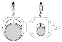
**3** Wrap the cable around the inside of the silicone case in the side slot. Wrap the cable around as many times as needed.
