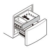
5 Replace the ice bin in the drawer. Insert the Durabase basket in the rail assembly.
