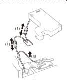
3 Rotate the hinge lever (1) clockwise. Lift the top hinge (2) free of the hinge lever latch.
