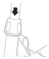
**6** Slide the steering clamp cover down and over the "E" shape fixed pin.
