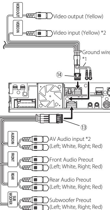
\*1 Secure the two ground wires together to the chassis of the main unit.
