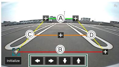
Make sure that lines **(A)** and **(B)** are horizontally parallel, and that lines **(C)** and **(D)** are of the same length.
