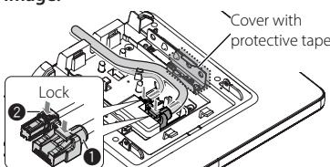
**2** Press and hold the display cable lock and then remove the cable.
