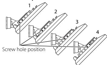
**6** Fix the display unit with four hexagon head screws (accessory ⑨).
