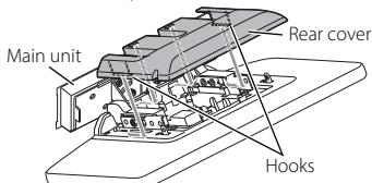
**9** Fix the display unit cover with two binding head screws (accessory ⑩).
