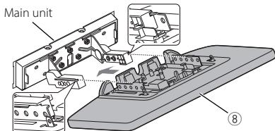
**5** Adjust the display height according to the screw hole position.
