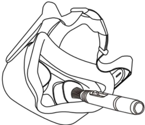
**3** Gently wipe the lens with the cleaning pad on the lens cleaning pen or with a cleaning wipes.
