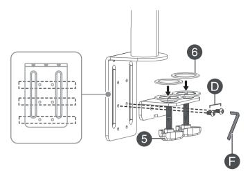
3 Slide the support base/base clamp assembly over the edge of the desk where you want your monitor mount installed, then tighten both base clamp screws by turning them counterclockwise. Make sure that the clamp assembly is flush with the desk to prevent wobbling.
