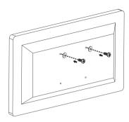
2 Lock the monitor plates into position with the 5 x 5 Allen wrench (**G**), then center the back of the first monitor on the monitor plate at the end of the monitor support bar.
