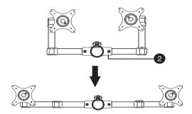
2 Slide the monitor support arm (2) over the top of the support tube (3). Make sure that the cable support brackets are installed and evenly spaced along the monitor support arm.
