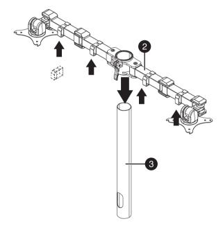
3 Tighten the monitor support lock when the monitor support arm is at the desired height.
