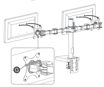
3 Align the mounting holes on the monitor with the holes on the monitor plate, then attach the monitor to the monitor plate using four screws (**A** or **B**) with washers (**E**). Tighten the screws firmly with a Phillips screwdriver, but do not overtighten. Repeat for the second monitor.
