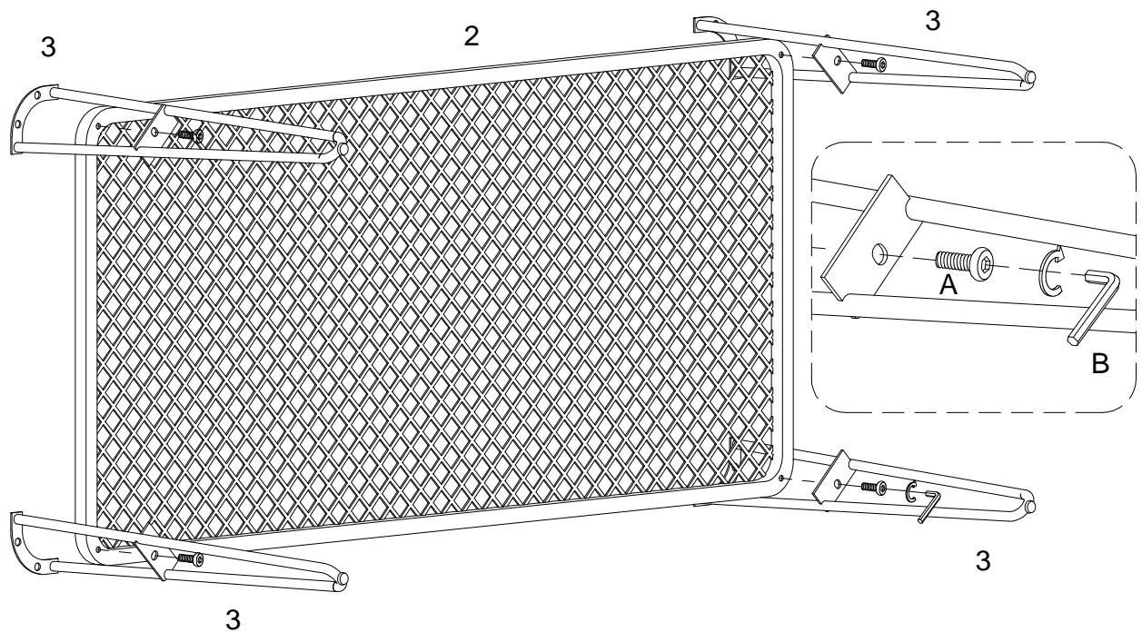
Attach part (3) to part (2) using bolt (A) with hex key (B).
