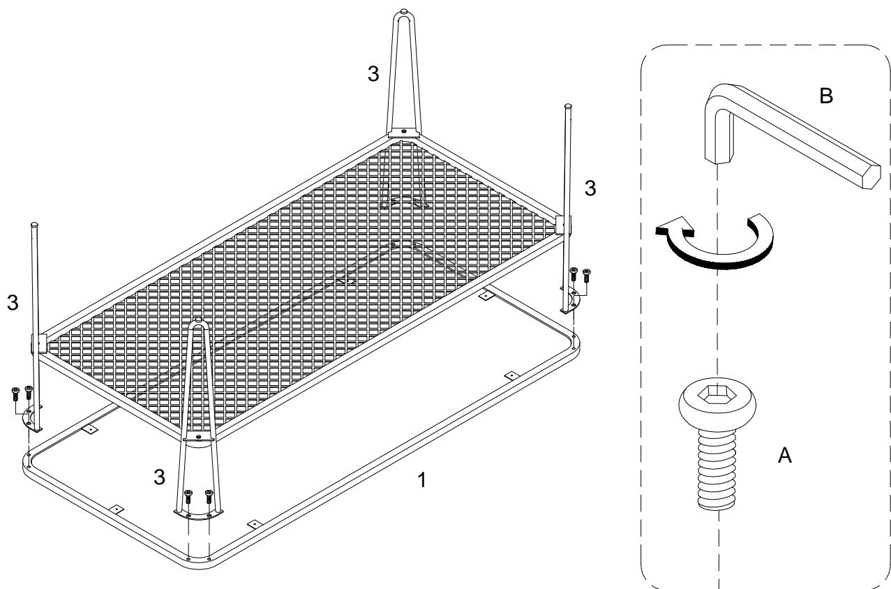
Attach part (3) to part (1) using bolt (A) with hex key (B).
