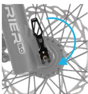
7. When you cannot screw the thru axle in any further, close the lever by folding it 180 degrees. There should be resistance building when the lever is closed, if there is no resistance repeat steps 5-7 again.
