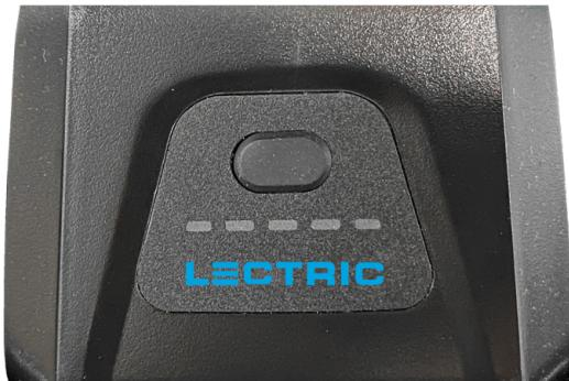
1. Hold down the
