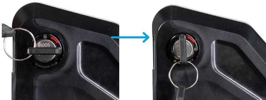
**NOTE:** Rear battery may be used with or without the front battery inserted. You may insert the battery with or without the keys in the battery. (If using dual batteries, insert the front battery before inserting the rear battery).
