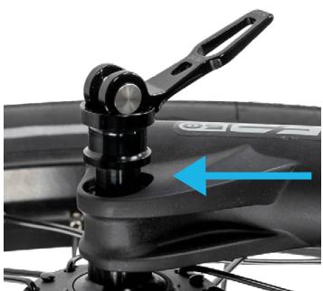
6. Align the quick release lever with the cutout in the thru axle endcap. Begin turning the lever clockwise, keeping the lever open and in the slot.
