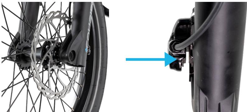
5. Slide the thru axle into the fork from the disc brake side. Push in until there is a firm stop and 0.25" gap between fork and thru axle endcap.
