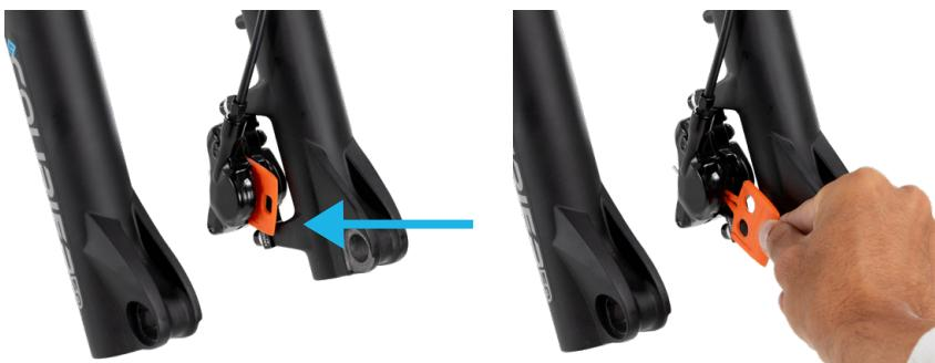
4. Install the front wheel by aligning the disc brake with the caliper brake pad slot.
