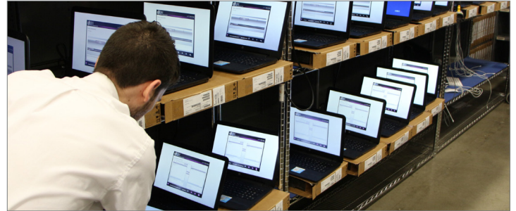
Geek Squad Agents installing custom configuration of software and imaging on multiple computers at one time.
