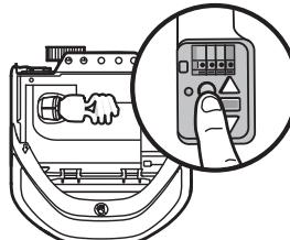
The lamp's light bulb will blink and the LED on the Smart Lamp Control will turn OFF when the device has been programmed.
