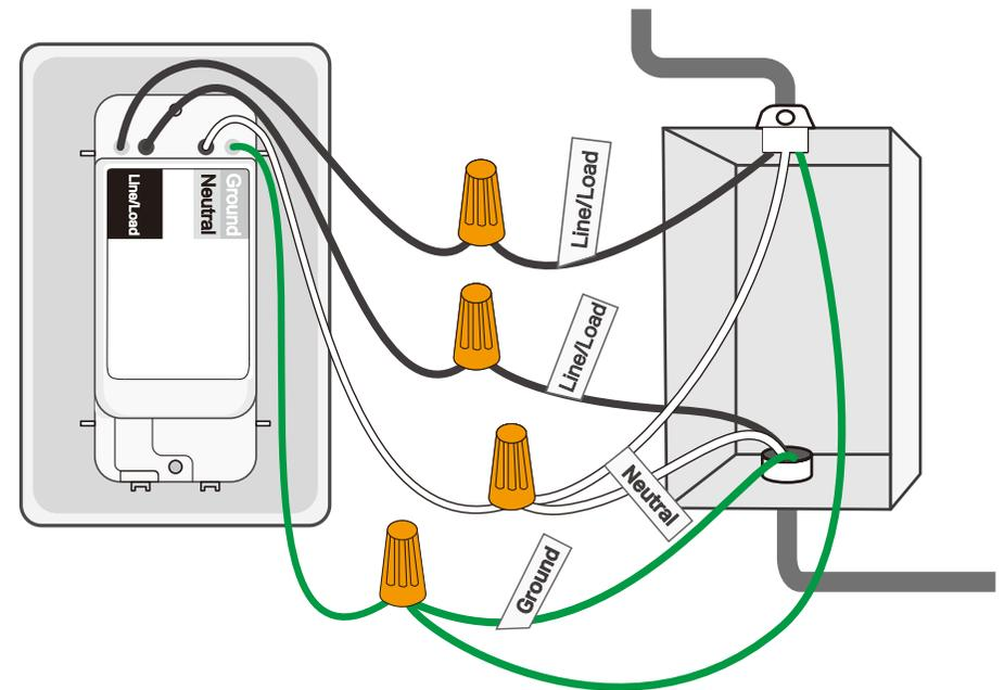
▀Note: No need to distinguish between Line and Load wires.
