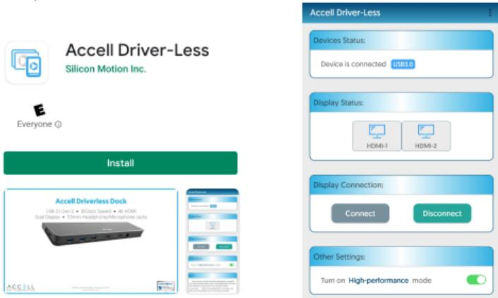
2. Connect the dock to your smartphone and launch the Accell Driver-Less App. The connected external monitor(s) will be enabled, ready for screen sharing and presentation.
