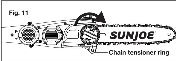
9. Raise the guide bar and tighten the end cover knob securely.
