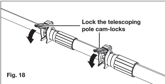
**WARNING!** Failure to lock the telescoping pole cam-locks as directed could result in personal injury.
