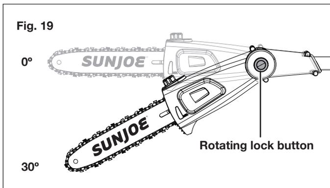
1. Rotate the pole saw head to the desired cutting angle while pressing the multi-angle head adjustment dial located on the back (Fig. 19).
