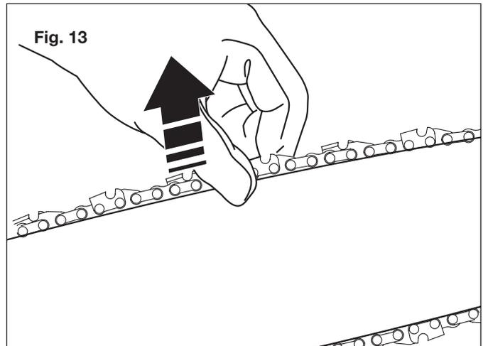
**NOTE:** If the chain is too tight, it will not rotate. Loosen the end cover knob slightly and turn the chain tension knob 1/4 turn counterclockwise. Lift the tip of the guide bar up and retighten the cover cap knob. Ensure that the chain can be rotated by hand without binding.
