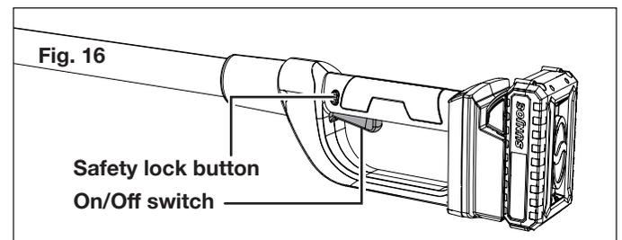
3. To turn the tool OFF, release the On/Off switch (Fig. 16).
