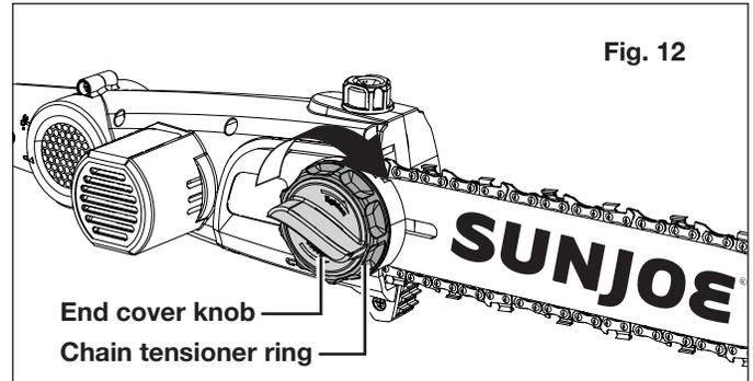
2. The tension is correct when the drive links on the chain do not slip out of the chain guide on the bar when the chain is pulled up from the middle of the bar (Fig. 13).
