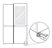
2 Open both doors and check to make sure that they close easily. If the doors do not close easily, tilt the refrigerator slightly more to the rear by turning both leveling legs to the left. It may take several more turns, and be sure to turn both leveling legs the same amount.
