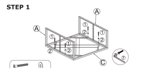
Please don't fasten the screw completely during assembly process, It will be likely to lead to an assembling problem that screw hole position is not aligned. You can fasten completely when all parts have been assembled.
