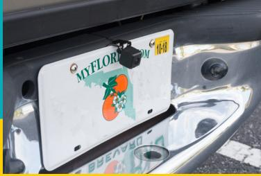
Relax in reverse. CAM-TGL features dynamic parking lines that move when you move. Simplifying maneuvering in even the most complex situations, the parking lines give you a clear understanding of the trajectory of your car before you reverse. The durable, water resistant camera features built-in motion sensors, once the vehicle starts moving the camera senses the movement and guidelines move to show the path of the vehicle.
