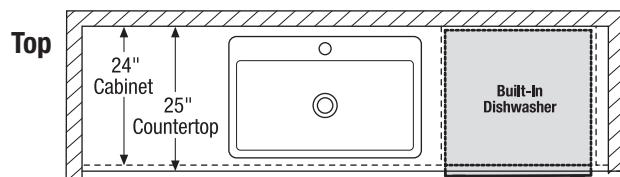
When installing appliance with sliding drawer or drop-down door directly across from obstructions, provide sufficient clearance for drawer extension or door swing.
