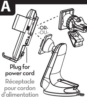
Join the device holder with the T-Notch on either the dash mount or vent mount. Slide until click. T-notch ball joint can be adjusted for best viewing angle.
