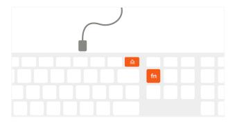
Press and hold one of the keyboard's Bluetooth keys for ~3 seconds, until the LED light starts to blink.
