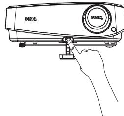
To retract the foot, hold up the projector while pressing the quick-release button, then slowly lower the projector. Screw the rear adjuster foot in a reverse direction.
