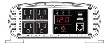
3. Once blue, the Low Voltage Alarm will be set to 10.5 Volts. The setting will not change when the inverter is turned off or the battery is disconnected (to go back to the default 11.5 Volt Low Voltage Alarm Setting, follow steps 1 and 2)
