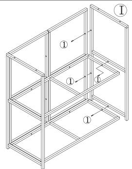
**STEP 8**Connect part from STEP 7 & Table Right Frame I (I) with Bolt (1)
