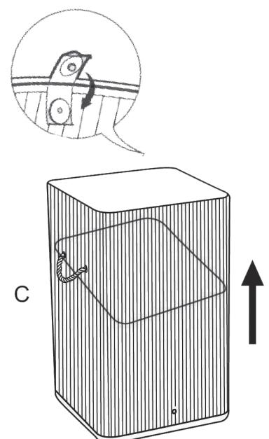
3. Fasten the metal frame with the interior clasps.
