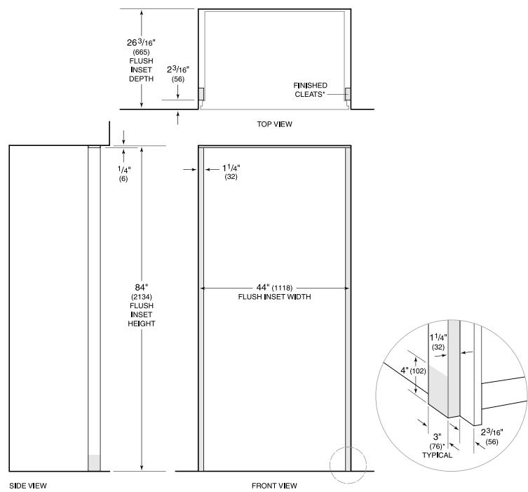
\*3" (76) typical depth. Shaded areas will be visible and should be finished to match cabinetry.
