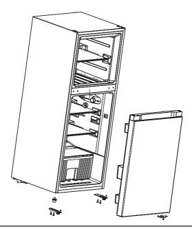
**6)**Place the refrigerating door from top to bottom, take out the gasket from the plastic bag in the instructions and put it into the axle hole on the left side of the refrigerating door, as shown in the picture. Fix the center hinge with screws and install the studs.
