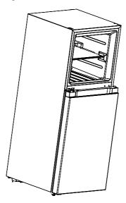
7) Put the freezer door on the middle hinge, assemble the upper hinge on the other side, fix the hinge cover on the upper hinge and fix hole cap on the other side.
