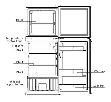
**Note:** To remove a refrigerator shelf, lift it up, then slide it out.
