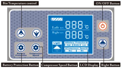
——Press the  $\triangle$  button or  $\nabla$  button to adjust the temperature the unit aims to achieve. Press the  $\triangle$  button to increase or the  $\nabla$  button to decrease the temperature.
