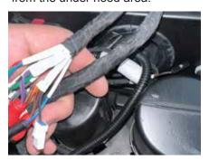
Once your main harness is in the dash cavity, take your radio harness and send the Pulse wires through the same grommet out to the under hood area.
