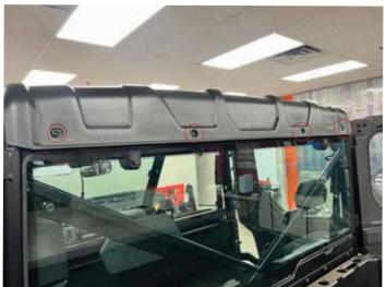
Pull back on rear bottom section of roof while lifting roof and resting on top of ROPS. Then push roof forward and remove.
