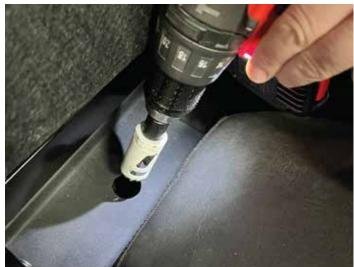
• Carefully route the wires through the hole and install the grommet after all wires are through.
