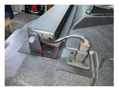
Bolt front roof section with (4) bolts into the rear cover panel and rear ROPS.
