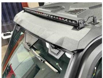
• Bolt front of roof loosely through the lightbar rear bracket hole.
