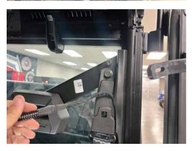
Remove (1) T27 bolt from front driver and (1) T27 bolt from passenger side of roof. Remove the speed clip under the roof (as it will not be needed anymore).
