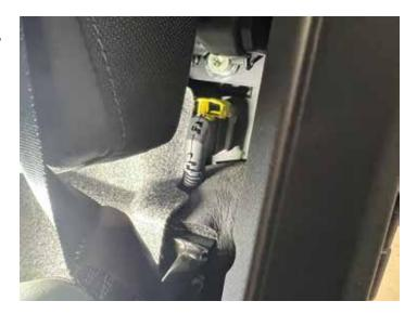
Disconnect power and ground terminals from Pulse network module using a 10mm socket.
