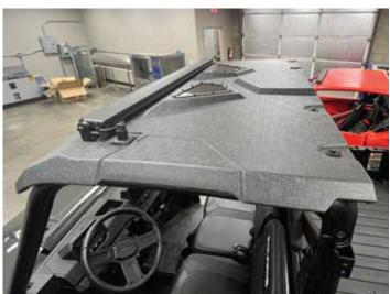
Run main audio roof harness down the passenger rear ROPS pillar and secure with (2) fir tree zip ties in the holes in the ROPS. Leave zip ties loose so you can adjust the wire length during install. You will tighten these later.
