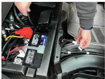
Run harness along factory wiring all the way up to the firewall. Zip tie to white tape marks.
