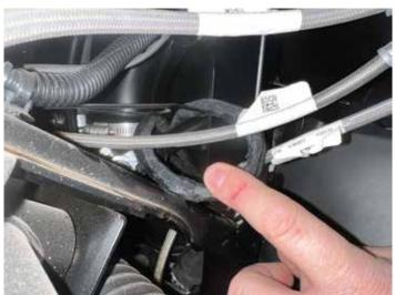
Pull the harness along the firewall and over the brake booster (avoiding all moving parts). Zip tie the harness to a vehicle harness or brake line away from moving parts. You will send it up through the hole where you can see the radiator fluid reservoir.
