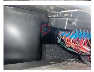
Disconnect air vents from front console then remove front floor console from vehicle.
