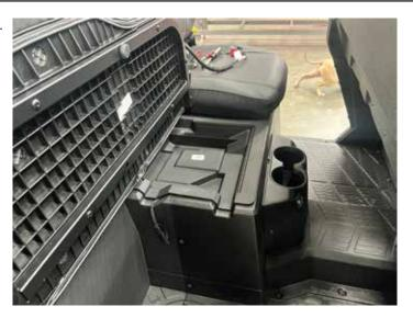
Remove (4) clips from passenger side of front console and (3) clips from driver side. There are (2) hidden clips in center console and if you have the Northstar model disconnect front AC hose. There is (1) clip hidden behind the fuse holder near the battery.
