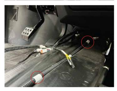
Run harness through firewall on the driver side of opening.
