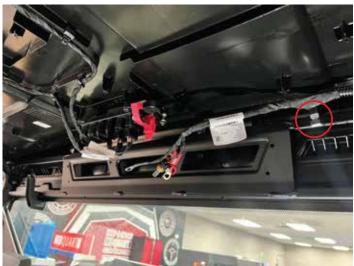
Pull harness out of rubber channel on rear pillar and remove from vehicle or tuck behind rear seat panel.
