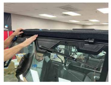
Press side foam up against front foam and run it along the ROPS toward the back.
