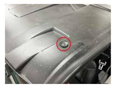
• Remove (4) T40 bolts from rear of roof.
