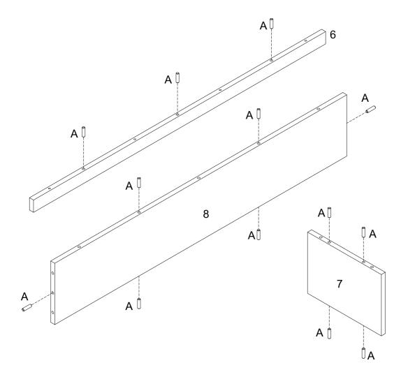
Insert wooden dowel (A) into parts (6,7,8) as per diagram.
