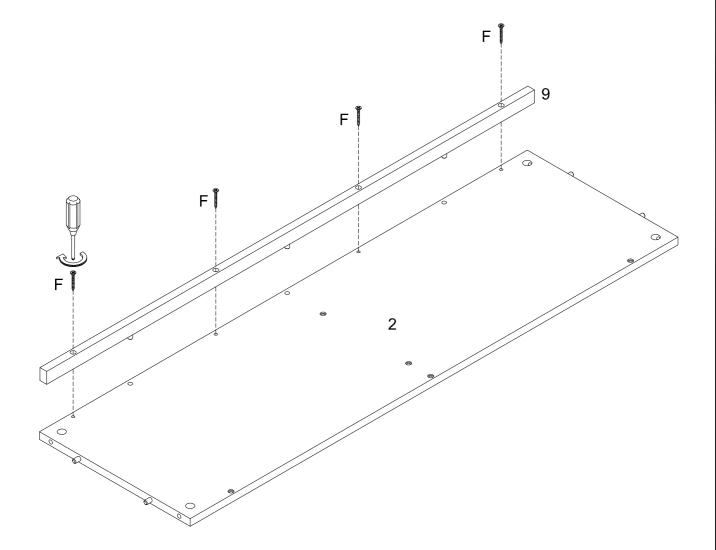
Using screw (F) attach part (9) to part (2) with Philips head screwdriver as per diagram.
