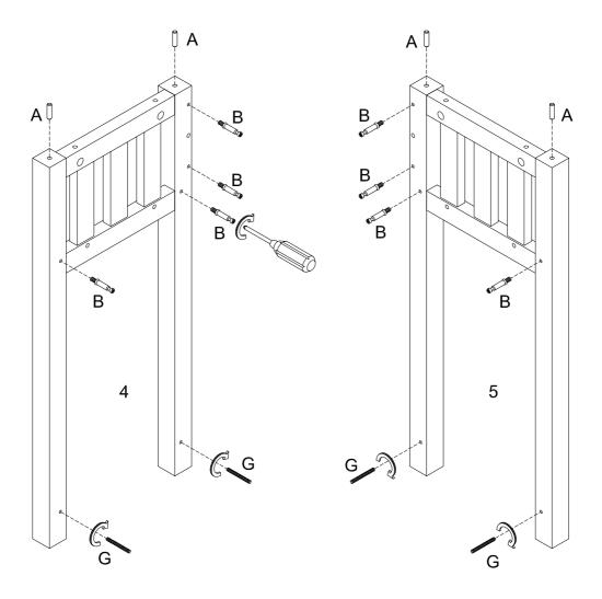
Insert wooden dowel (A) into parts (4,5). Secure cam bolt (B) to parts (4,5) with Philips head screwdriver. Secure bolt (G) to parts (4,5) as per diagram.
