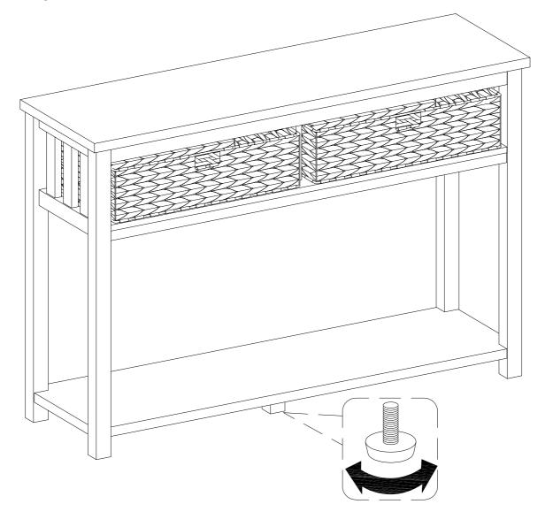
Position the assembled unit at the desired location, if necessary adjust the floor leveler at the bottom of the support leg to level the unit.
