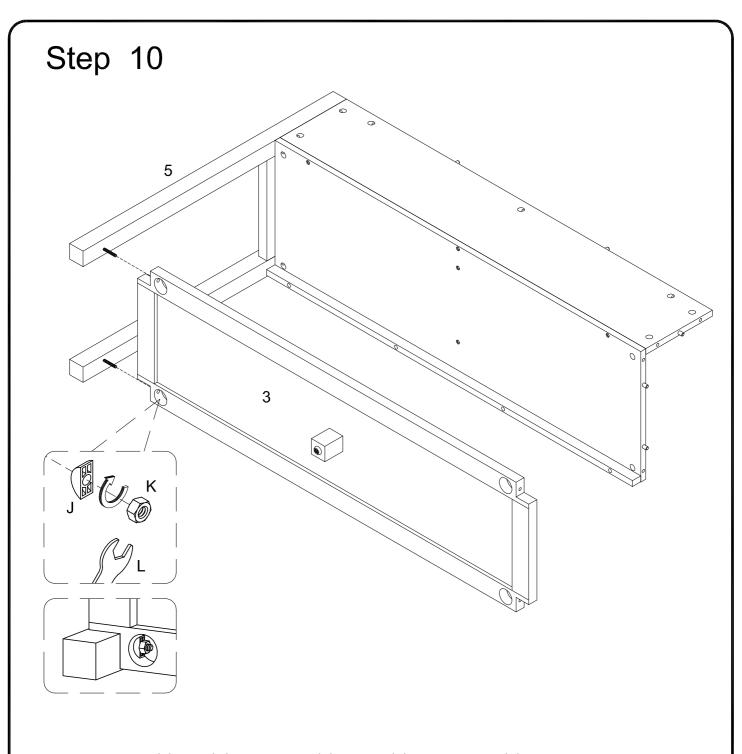
Using washer (J), nut (K) attach part (3) to part (5) with wrench (L) as per diagram.
