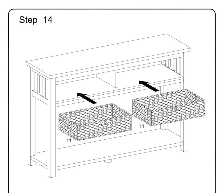
Put part (11) into unit as per diagram.
