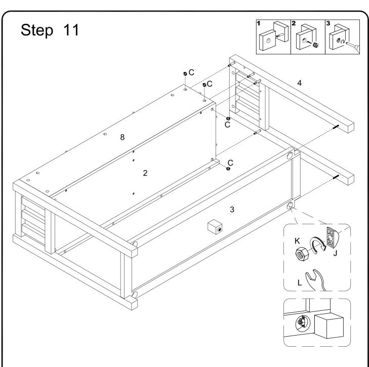
Using cam lock (C) secure parts (2,8) to part (4), then using washer (J), nut (K) attach part (3) to part (4) with wrench (L) as per diagram.
