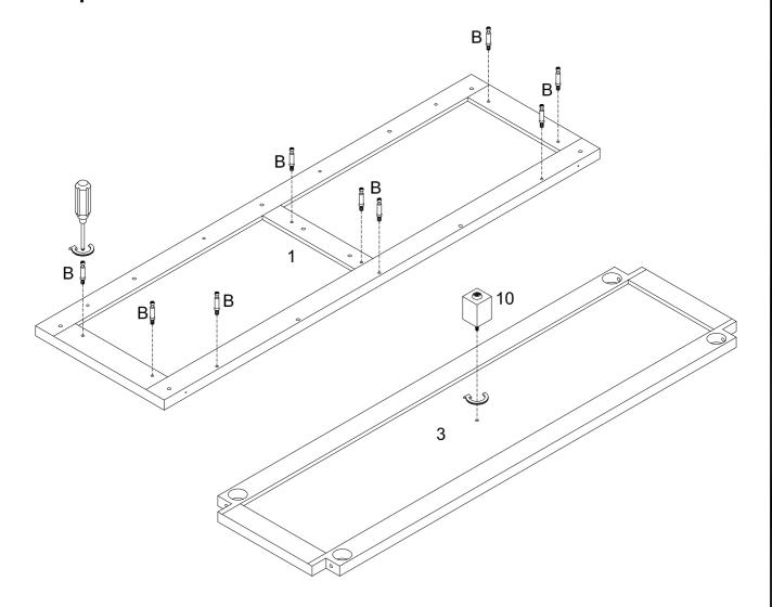
Secure cam bolt (B) into part (1) with Philips head screwdriver; Attach part (10) to part (3) as per diagram.
