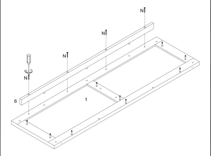
Using screw (N) attach part (6) to part (1) with Philips head screwdriver as per diagram.
