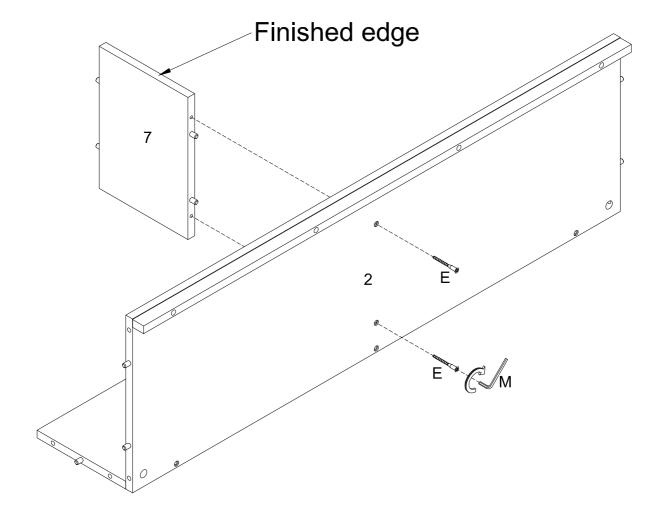
Using screw (E) secure part (2) to part (7) with hex key (M) as per diagram.
