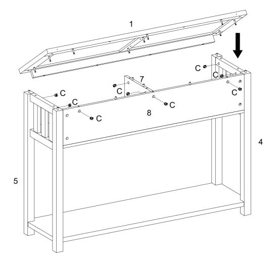
Using cam lock (C) secure part (1) to parts (4,5,7,8) with Philips head screwdriver as per diagram.
