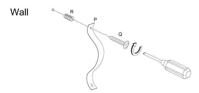
Using screw (Q) attach Velcro strap (P) into Nut (R) to wall with Philips head screwdriver as per diagram.
