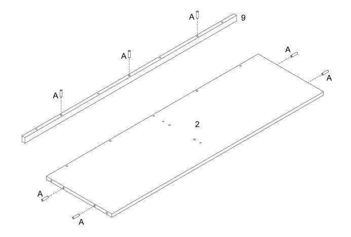
Insert wooden dowel (A) into parts (2,9) as per diagram.
