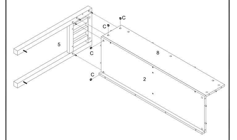
Using cam lock (C) secure parts (2,8) to part (5) with Philips head screwdriver as per diagram.
