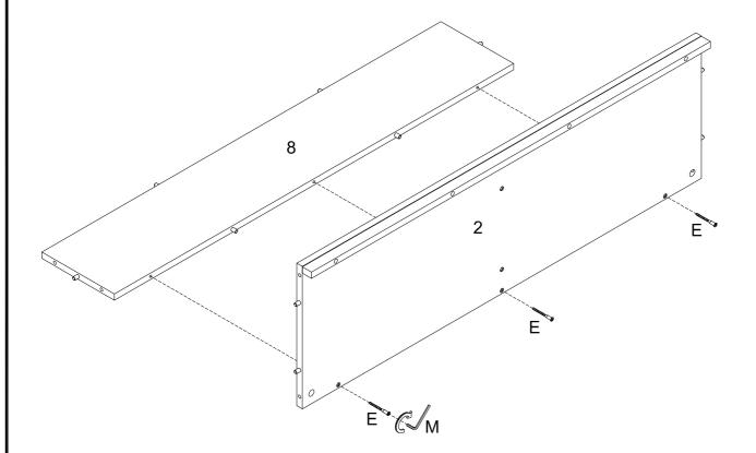
Using screw (E) secure part (2) to part (8) with hex key (M) as per diagram.
